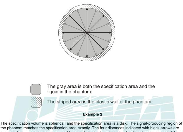
the phantom matches the specification area exactly. The four distances indicated with black arrows are measured on the image and compared to the actual phantom diameter. Additional measurements (shown by gray arrows) are suggested. A central pin in the phantom is useful, but not essential, for ensuring that each of the measurements represents a diameter.
