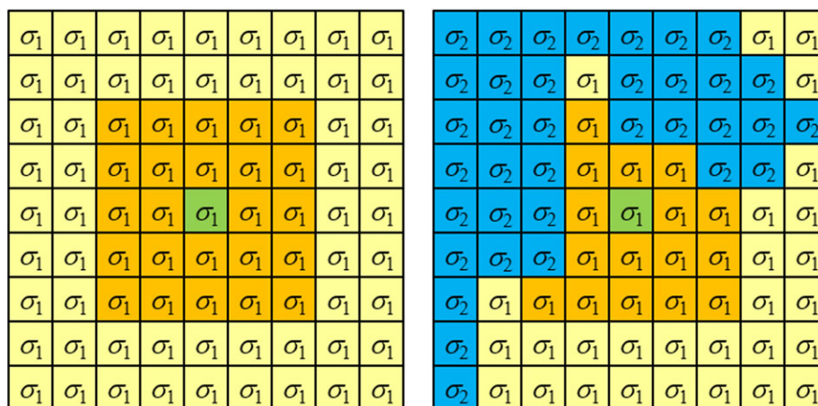
FIGURE 3 Illustration of bilateral filtering in two spatial dimensions. Left: In a homogeneous tissue with conductivity \sigma_1 , the filter kernel (orange voxels) around the target voxel (green) has its predefined maximum size (here, 5 \times 5 voxels). Right: At the boundary between two tissues (having yellow and blue conductivities \sigma_1 and \sigma_2 , respectively), the filter kernel is restricted to voxels having the same conductivity, i.e. belonging to the same tissue type. Typically, tissue type is identified from an independent magnitude image
